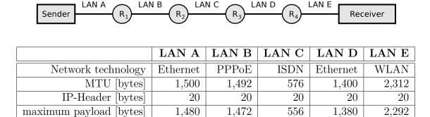
Display graphically the way, the payload is fragmented, and how many bytes of payload each fragment contains.
