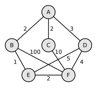
2. Calculate the shortest path from node A to all other nodes using Dijkstra's algorithm.
